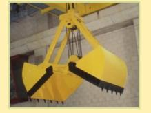
2. Lifting and lowering of the closed orange peel grab or grab. When the teeth or blades are already closed, if the closing rope is still pulled the grab goes up. So, in order to avoid that the holding rope remains too loose it must be wound in a simultaneous way as the closing and lifting.
