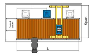
It is important to define the orange peel grab resting area, the EOT crane parking area, the length to pick up the rope-holder carriages and that the installations have an access for crane maintenance.
