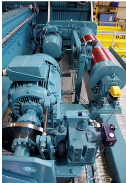
6E - Open winch with double planetary gearbox double drum and safety brake drum
