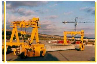
HANDLING OF CONCRETE BEAMS
