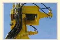
Hydraulic lifting and direction motors for the crab, independent for each function
